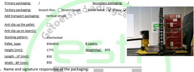
8. Test conditions: Relative humidity: 48% - Temperature: 2°C - Sliding of the pallet is prevented mechanically.
