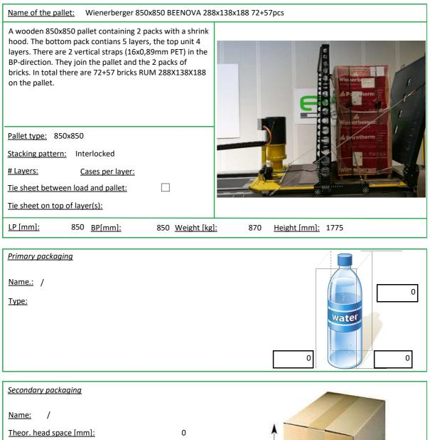
Gross weight [kg]: Compression force [N]: Fluting type: Prim units per sec. unit:
